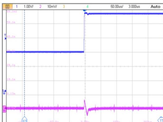
Fig.12 Line Trans 3.8V~5.5V
