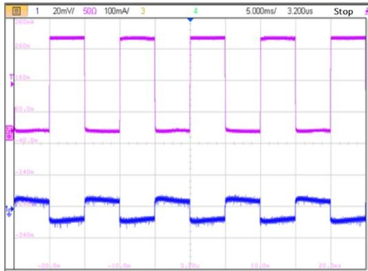
Fig.10 Load Trans 1mA – 300mA ( $V_{OUT} = 2.8V$ )
