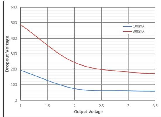
Fig.3 Output Dropout Voltage vs. Load Current (VOUT=2.8V)
