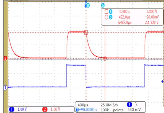
Fig.9 Load Trans 1mA – 300mA ( $V_{OUT} = 1.8V$ )
