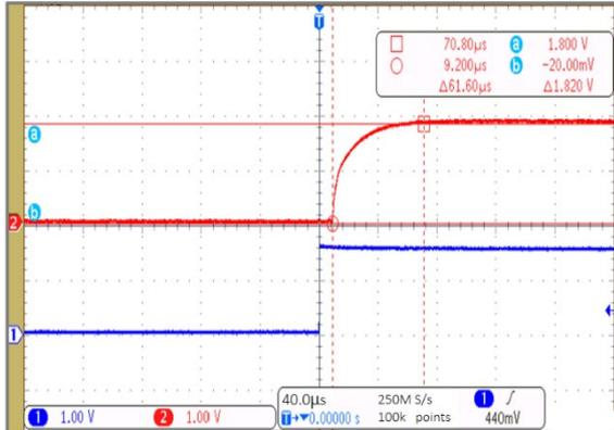
Fig.8 EN Shutdown ( $V_{OUT} = 1.8V$ )
