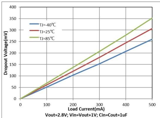
Fig.4 Dropout Voltage vs. Load Current (VOUT=1.8V)
