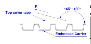
The force for tearing off cover tape is 10 to 130 grams in the arrow direction under the following conditions (referenced ANSI/EIA - 481 - D - 2008 of 4.11stadnard).
