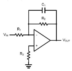
Figure 4. Low Pass Active Filter
