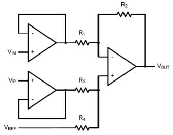
Figure 5. Instrument Amplifier
