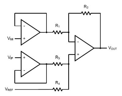
Figure 5. Instrument Amplifier
