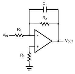
Figure 4. Low Pass Active Filter
