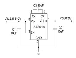
Figure 1. Basic Application Circuit with A7801A
