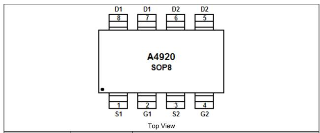
Pin# **Symbol Function** 1 S1 Source 1 2 G1 Gate 1 3 S2 Source 2 4 G2 Gate 2 5 D2 Drain 2 6 D2 Drain 2 7 D1 Drain 1 8 D1 Drain 1
