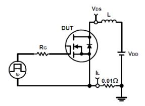
Switching Time Test Circuit and Waveforms
