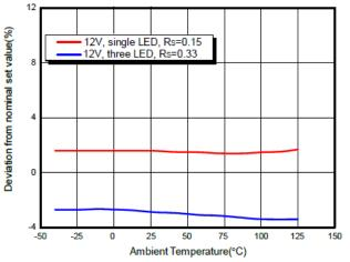
20. Voltage across  $R_{\text{SENSE}}$  vs. Temperature L=47uH
