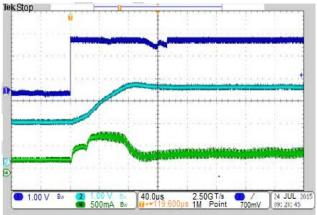
6.  $V_{IN}$ =3.3V,  $V_{O}$ =5.0V,  $I_{O}$ =0-0.5A
