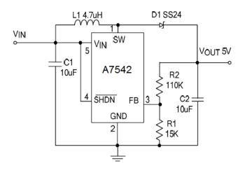
Figure 1. Basic Application Circuit with A7542
