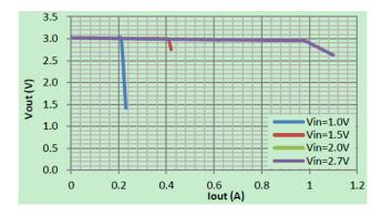
Output Voltage vs. Output Current 4. (Vout=3.3V)
