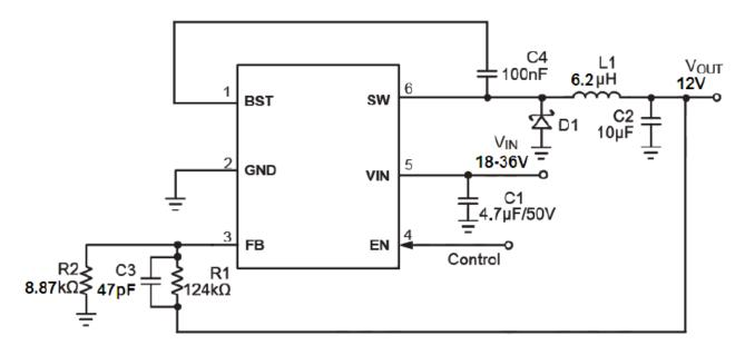
12V output typical application circuit
