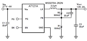
Figure 1. Typical Application Circuit
