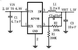
Figure 3. Circuit of Adjustable Output Version
