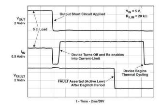
6. No Load To Short Circuit Transient Response
