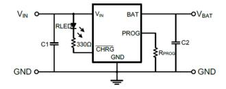
NOTE: C1=4.7uF, C2=10uF,  $I_{BAT}$ =( $V_{PROG}/R_{PROG}$ )\*1000
