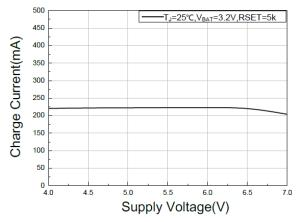
Charge Pin Current vs. Charge Voltage (Weak Pull-Down State)
