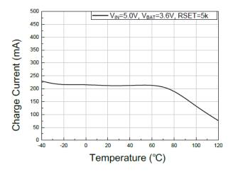
14. Charge Pin Current vs. Temperature
